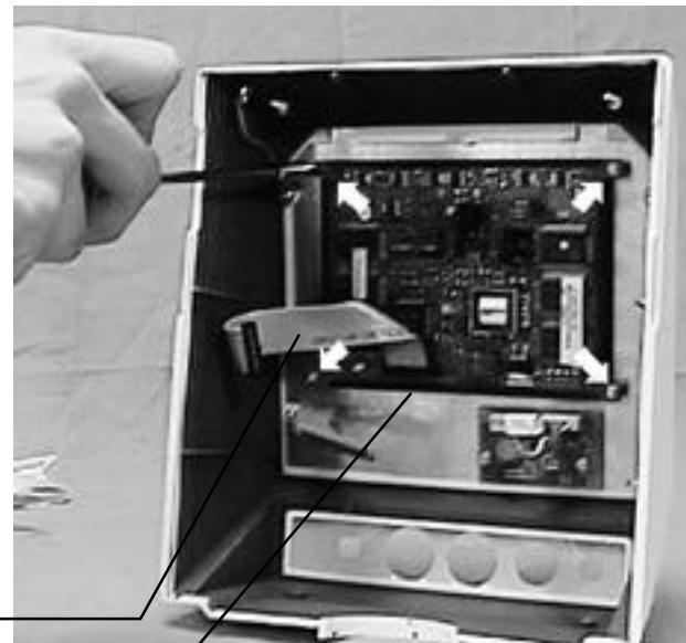
e) To separate the LED's board, remove the two nuts (3) and spring washers. Under this board there are two nylon nuts placed as spacers.
