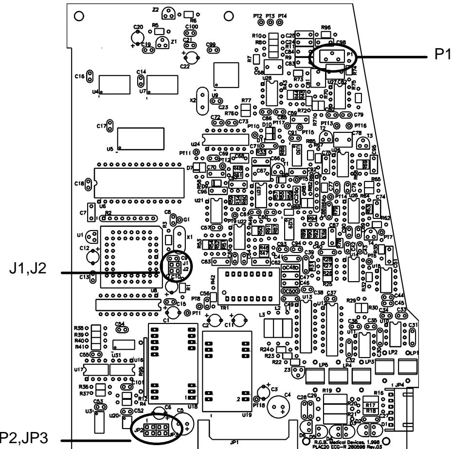
The potentiometer P1 is used to adjust the notch filter (50 or 60 Hz). The signal can be watched in PT3 with an oscilloscope.
